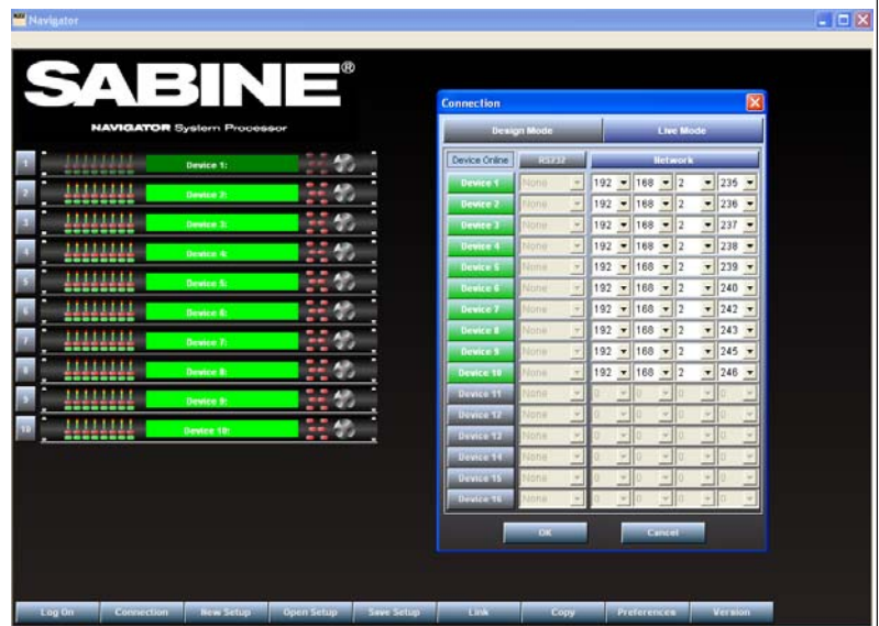
Main screen in Navigator Software, showing Connection window with IP addresses assigned and 10 devices present. Device 1 is not connected.
